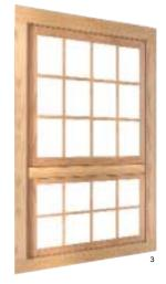
Attach interior wood muntin bars to window glass with clear 3M™ Dual Lock™ Low Profile Reclosable Fasteners.
