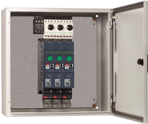
Example of GV2/ATV320 direct mounting in an enclosure: GV2L circuit breakers + GV2454 and GV2G05 accessories + ATV320U15N4B drives
