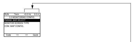
**[PARAM. BAR SELECT]**: Selection of 1 to 2 parameters displayed on the top line (the first 2 cannot be modified).
