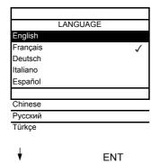
Display after the graphic display terminal has been powered up for the first time. Select the language and press ENT.
