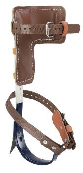
Klein's Pole Climber set includes the pads, steel sleeves, leg irons, gaffs, split rings and nylon calf and ankle straps. The secure sleeve and leg iron connections are adjustable. Contoured leg irons help position gaffs securely and comfortably. The replaceable gaffs firmly attach to the leg iron with a center pin and two TORX® screws. High-grade leather climber pads are cushioned for maximum comfort.
