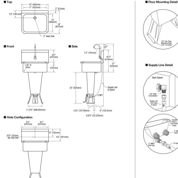
.375" dia. Floor Mounting Holes 4.25" on Center Supply Line Detail Back Splash Π Ŵ Double Knee or Foot Pedal Valve .5" MNPT Inlet Hot To Spour
