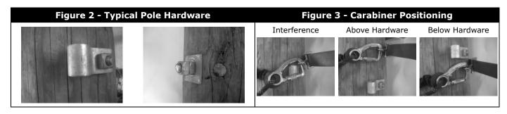
Although it is extremely unlikely that such a condition will result in a fall hazard, linemen need to be aware of the potential for this type of interaction with the captive eye carabiner.
