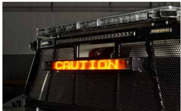
MB1 mounted on a HRX Series Headache Rack installed on a Chevrolet Silverado
