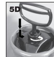
**TO UNLOCK PUMP:** Turn handle counterclockwise until 3-prong clamp is loose. Then rotate clamp counterclockwise to stop and lift out.
