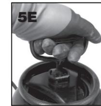
**TO RELEASE HANDLE:** Push down to depress coil spring and turn handle counterclockwise 1/4 turn, then lift handle.
