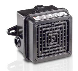
Model 350WBX (AC current) Vibratone® horn produces sound by electro-mechanical vibration of a stainless steel diaphragm. The horn mechanism with diaphragm is attached to the grille. The water- and dust-tight backbox is ideal for indoor or outdoor use.
