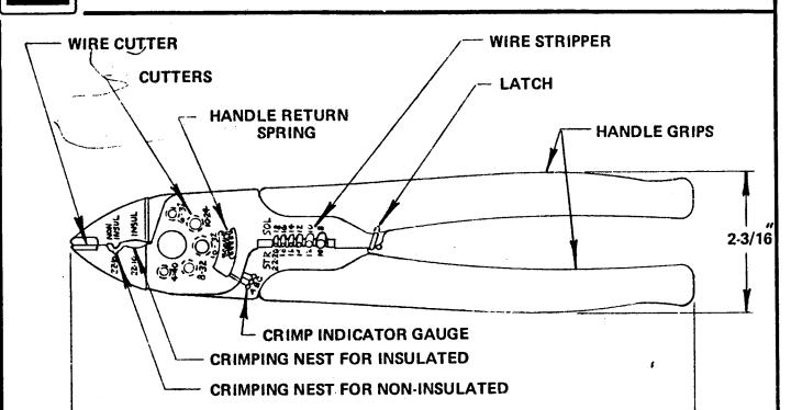
WIRE CUTTER - FOR NO. 10 AWG & SMALLER SOLID OR STRANDED WIRE.
