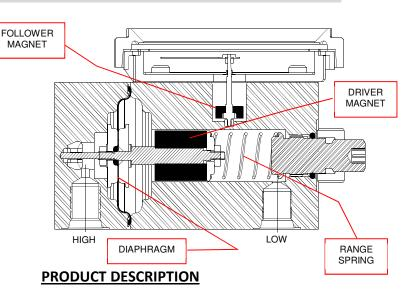
The Model 142 "Delta Meter" is a differential pressure instrument available as a switch, gauge, or both. A flexible elastomer diaphragm and calibrated range spring are moved by differential pressure. A magnet, coupled with the diaphragm, transmits motion through the wall of the pressure housing to a follower magnet attached to an indicating pointer. The rotation of the follower magnet causes the pointer to track movement of internal
