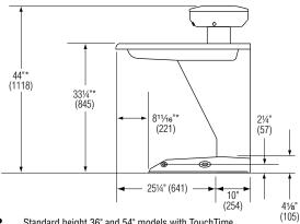
Standard height 36" and 54" models with TouchTime, infrared, or air metering hand activation are ADA/TAS compliant when mounted at standard height dimensions. Juvenile height 54" model with TouchTime, infrared, or air metering hand activation is ADA/TAS compliant.
