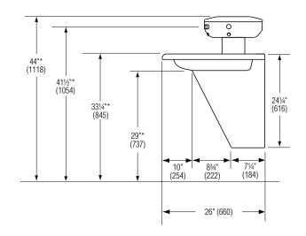
Wall mounted 54" and 36" models with TouchTime, infrared, or air metering hand activation are ADA/TAS compliant when mounted at standard height dimensions. Wall mounted 54" model with TouchTime, infrared, or air metering hand activation is ADA/TAS compliant when mounted at juvenile height.
