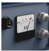
Each Kraftform Kompakt VDE set has been tested individually at 10,000 volts, in accordance with IEC 60900.This ten-times-higher testing load guarantees safe working at their maximum permitted load of 1,000 volts. Handle/interchangeable blade system
