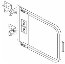
STEP 1. Attach angle iron adapter bracket to the Ladder Safety Gate mounting bracket with provided bolt.
