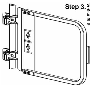
STEP 3. Adjust the Ladder Safety Gate so the top of the gate is 42' above platform/walking surface. Tighten all bolts.
