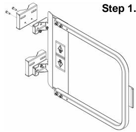
**STEP 1**. Attach Large Pipe adapter bracket to the Ladder Safety Gate mounting bracket with provided bolts.
