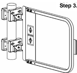
Step 3. STEP 3. Adjust the Ladder Safety Gate so the top of the gate is 42' above platform/walking surface. Tighten all bolts. If more than 1/4" of thread extends past the nylock nut, trim to 1/4".
