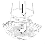
2. Slide HEPA filter element down over filter frame. Ensure filter is centered over the Velo air intake.
