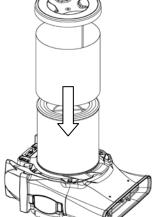
filter assembly and tighten with wingnut. This will lock the filter assembly snugly to the airmover Do not overtighten
