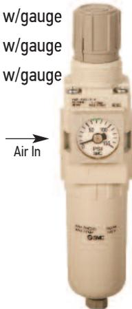
"High Pressure" air filter/regulators and lubricators are necessary when air pressure supplying these devices exceeds 150 PSI, which is the maximum pressure rating for the normal "Low Pressure" filter/regulators. This is the case if you are using a two stage air compressor which typically has a pressure of 220 - 250 PSI.
