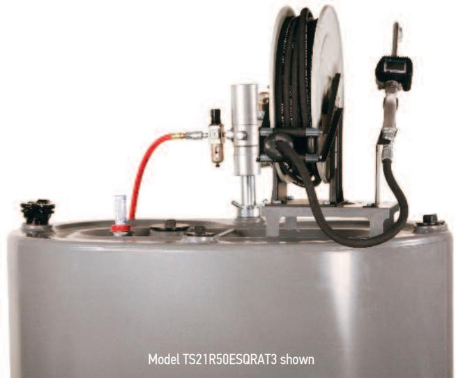
**Example:** Tank system w/3:1 pump, 25' reel, electronic meter w/quart cal., rigid spout, auto non drip tip and 275 gallon oval tank. System comes complete with foot valve, 2" bung adapter, air filter/regulator, air coupler set, 1/2" x 2' oil connection hose, 3/8" x 6' air connection hose, tank gauge, vented fill cap.
