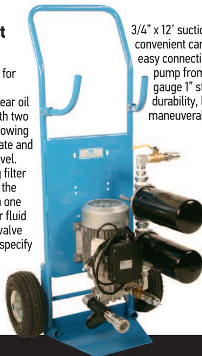
3/4" x 12' suction and discharge hoses are included and have convenient cam and groove couplings at each end to allow easy connection/disconnection. An inlet strainer protects the pump from damage. The Cart is constructed of heavy gauge 1" steel tubing for strength and powder coated for durability, large 10" pneumatic tires provide easy maneuverability.
