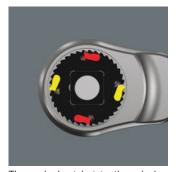
The dual-ratchet-teeth design means that a 76 fine-toothing division can be achieved from the 38 robust teeth with a return angle of only 4.7°.
