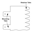
1.Temporarily secure wrap strips to pipe with masking tape. Measure and cut collar to length, providing a 1" (25 mm) overlap.
