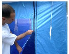
To deflate unit, make sure the entrance and exit doors are unzipped and rolled up.
