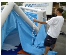
The FSI shelter will rapidly deflate (within 1 minute or so). As the unit collapses, each person should pull inwards on the
