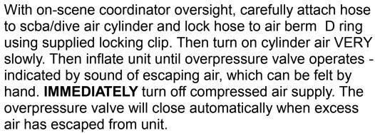
NOTE! Never cover/block the overpressure valve, as the unit may burst!
