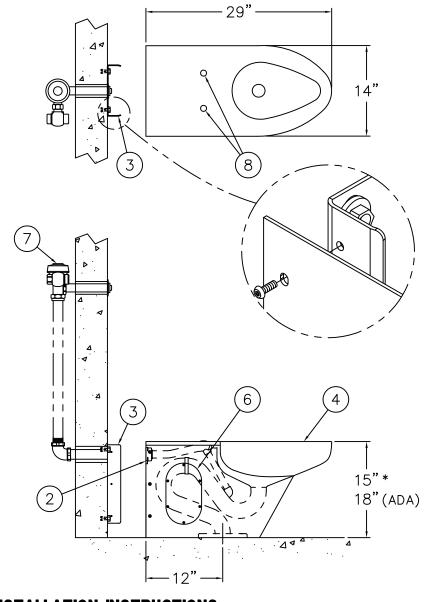
NOTE: USE ONLY APPROPRIATE UPC/CUPC CERTIFIED FLUSH VALVE FOR THE INSTALLATION OF THIS TOILET.
