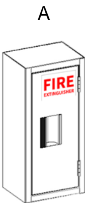
Fire Extinguisher Cabinet
