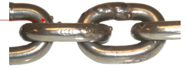
THE DAMAGE: Gouged links
