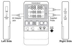
Probe labeled P1 must be plugged into the probe jack labeled "P1" and probe labeled P2 must be plugged into the probe jack labeled "P2".
