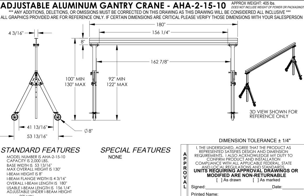
92" MIN LEAD TIME WILL START UPON RECEIPT OF SIGNED APPROVAL DRAWING 122" MAX DISTRIBUTOR'S NAME: HEIGHT IS ADJUSTABLE IN 6" INCREMENTS CASTERS: (4) Ø8" X 2" WIDE GLASS FILLED W.O.# X VESTIL MANUFACTURING NYLON SWIVEL CASTERS WITH FOUR DRAWN BY: ND LOCKING POSITIONS DATE: 01/08/08 SALES: X CRANE MAY BE TAKEN APART AND BUNDLED WITH reference: X SCALE: 1:34 FILE NAME: (2) INCLUDED STRAPS FOR EASY TRANSPORT ALUMINUM CONSTRUCTION QUOTED LEAD TIME: Y QUOTE # 28-007-194 Χ
