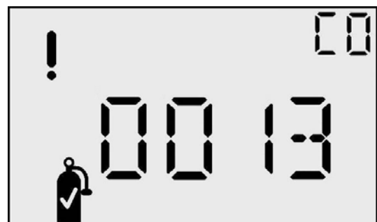
Spanning Failed Screen
