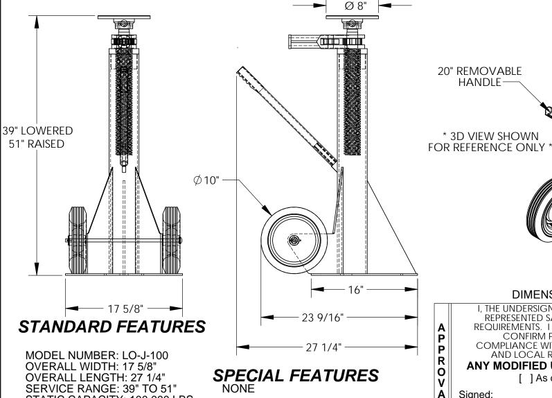
STATIC CAPACITY: 100,000 LBS. LIFTING CAPACITY: 50.000 LBS.
