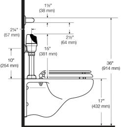
WHEN INSTALLING IN A HANDICAP STALL: Per the ADA Guildlines (section 604.9.4) it is recommended that the grab bars be split or shifted to the wide side of the stall. If grab bars must be present over the valve, use the alternate ADA installation as shown to the right.
