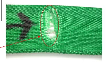
THE DAMAGE: Holes/Snags/Pulls exposing internal core yarns
