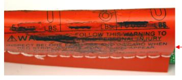
THE DAMAGE: **Illegible or Missing Tags** – The information provided by the sling tag is important for knowing what sling to use and how it will function.
