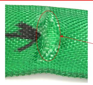
THE DAMAGE: Cuts to the cover NOT exposing internal core yarns – Tuflex roundslings all have a double walled jacket protecting the inner core yarns from damage. If damage (except for chemical or heat) appears only to the outer jacket and does not expose the inner core yarns, the sling may remain in service. To extend sling life, the sling may be returned to Lift-All for inspection and application of a patch to cover the damaged area.
