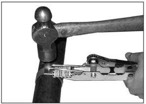
**3.** Place punch on clamp and while holding tension with ratchet wrench, lock clamp by striking punch once or more with hammer, depending on object being clamped.
