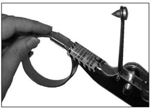
1. Tool is designed specifically for 3/8" and 5/8" center punch clamps only. Insert clamp in tool and then insert wrench assembly. If you prefer, install wrench assembly before clamp is inserted. Slot must be aligned with clamp tail.
