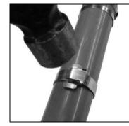
8. Hammer down buckle ears to complete BAND-IT clamp.
