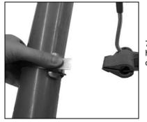
7. Remove tool, holding stub of band down with thumb.
