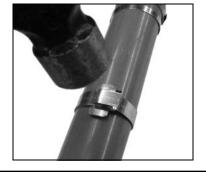
8. Hammer down buckle ears to complete BAND-IT clamp.
