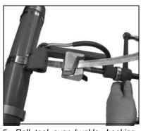
5. Roll tool over buckle, backing off with tension handle 1-1½ turns throughout entire rolling operation. Failure to back off tension with tension handle throughout entire course of rollover may result in breaking of band. There is no loss of tension as band released is used up in the bend.
