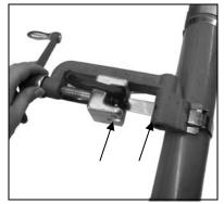
3. Place band in opening of tool nose and gripper block. Move into slot as far as possible, to avoid buckle sliding into tool nose. Tighten band clamp by turning the tension handle clockwise while holding band gripper tight against band. NOTE: The spring load of the band gripper is not intended to secure and prevent the band from slipping during tension process.
