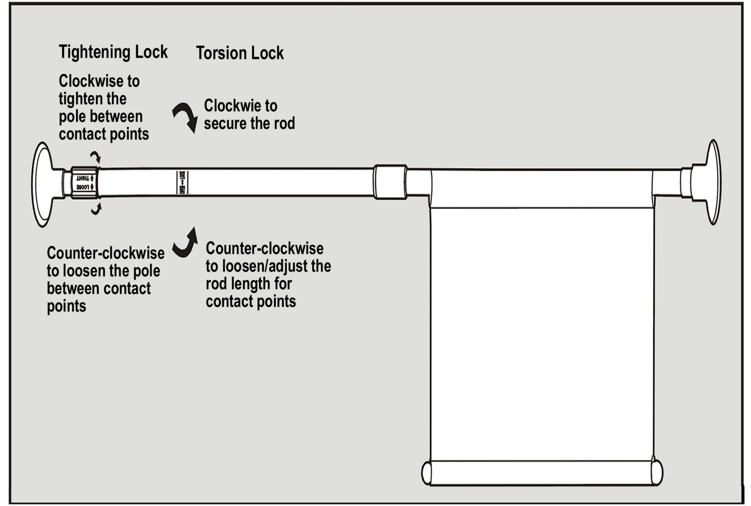
Expand the extendable pole assembly to the approximate doorway or hallway opening. Secure the Torsion Lock with a clockise turn. Turn the Tightening Lock clockwise to secure the pole assembly between the contact points.
