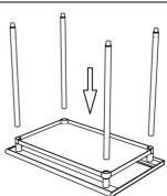
2. Insert 4 legs (B) into sockets. Fix them with the set screws (not too tight).
