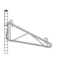
1. Select desired height, mark location of the bottom shelf on each post, and snap tapered Plastic Sleeves(C)(With tapered side facing up), to marked grooves on each support post. 2.Place Wall Mount Bracket (D) at top of each Support Post (A) and guide down to tapered Plastic Sleeve(C). Each Shelf Mount Bracket will level others when snug over Plastic Split Sleeves (C)
