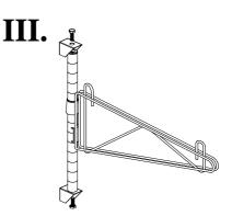
3. Measure the wall where the shelving is to be installed. Using the proper hardware (Not included) for the type of wall you are mounting to, secure the top bracket (E) as shown. Secure Both ends of support post (A) and then secure bottom bracket (E). Repeat Process with each support and bracket assembly.
