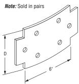
11 Gage Steel, 0.125" Aluminum 3/8"-16 spline bolts & flange nuts furnished.
