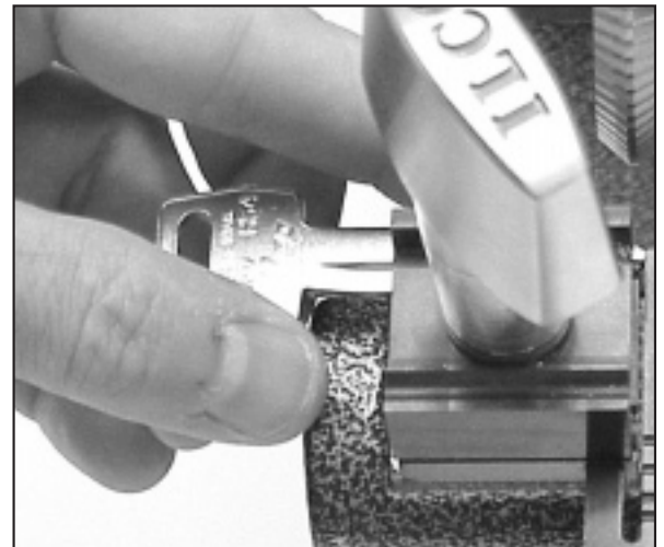
Align key using shoulder gauge or correct tip stop as required
