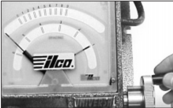
Rotating Spacing Crank to center Spacing Needle over desired cut position
