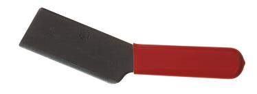
The Klein Tools Bell-System Cable-Sheath Splitting Knife features a heavy-duty forged steel blade perfect for cutting cable sheaths with its chisel-like edge. The handle is plastic-coated for more comfortable handling.
