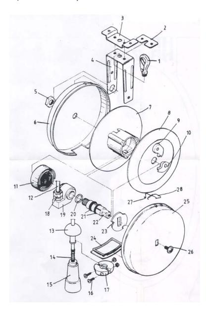
2 Locking Piece Assembly Piece 3 Assembly Frame 4 5 Hexagonal Screw Outer Shell 6 Wheel Disc seat 7 Wheel Disc Cove 9 Snap Tooth 10 Snap Tooth Spring Sheet 11 12 Air Tube 13 Fixing Rubber Ball Spring Sheet 14 **Protective Casing** 15 16 Screw Fixing Clamp Piece 17 Air Intake Screw 18 19 Calve Seat 20 Washer 21 O-ring 22 Wheel Core 23 Snap Tooth Block Guide Piece 24 25 Outer Shell 26 Screw 27 **Auxiliary Sling Valve** 28 Fastening Piece
