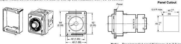
Note: Recommended panel thickness: 1 to 3.2 mm.
