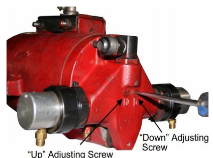
Figure 3 -Hoisting and Lowering Speed Adjustment
