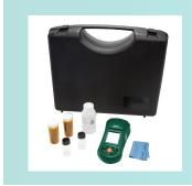
Meter comes complete with all the accessories to conveniently test the turbidity of municipal water, food and beverage water, and other aqueous solutions where fluid clarity is important. Portable design allows you to take measurement on-site instead of bringing solution back to the lab. Measures up to 1000 NTU (Nephelometric Turbidity Unit) with 0.01 NTU resolution.
