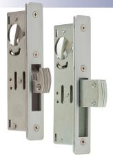
360° turn of the key or thumbturn retracts the bolt. The bolt provides maximum security on single leaf aluminum stile doors and will retrofit to existing locks previously installed. Accepts standard 15/32" (29.4 mm) diameter mortise cylinder or thumbturn with AR cam. Available with straight bolt (185) and hook bolt (HB185).
