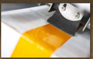
Delivers full utilization of the tape's adhesive via multiple, flexible wipe-down mechanisms, resulting in increased fiber tear for tamper evident security; even on under-filled cartons.
