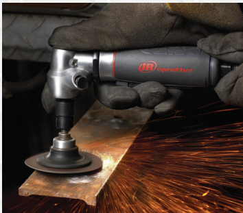
Grinding and Descaling
