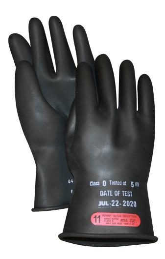
These rubber insulating gloves protect against electrical shock and should be tested every 6 months in accordance with ASTM F496, "Standard Specification for In Service Care of Insulating Gloves and Sleeves" at an authorized safety equipment testing facility. Type I natural rubber. Meet ASTM D120, IEC EN60903, and NFPA 70E standards.
