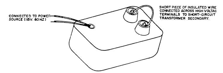
8. Such a short circuit will remove the hazard of shock and will not harm the transformer in any way. It has been designed to have a short circuit current limited to 23 ma which is very close to its normal operating current.
