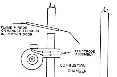
If a spark does exist and the nozzle is not plugged, the electrodes can be out of position. Check and adjust, including the correct gap width 1/8" to 5/32". These can most accurately be spaced by using a 1/8" or 5/32" feeler gauge.
