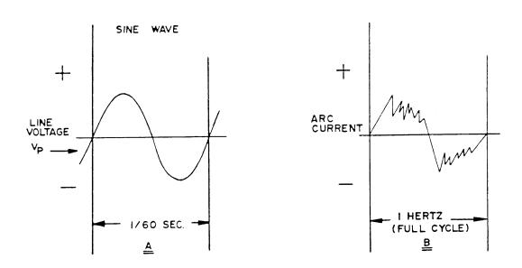
When a spark or arc is established across the electrode gap the current through this arc is no longer a smooth sine wave, but is an erratic shape that has a very large quantity of small "Spikes" or harmonics. You can get an idea of this phenomenon by listening to the buzz sound of an electrical arc. (Drawing B above).
