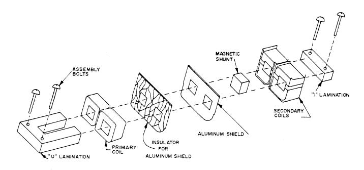
Most North American ignition transformers have been built to operate continuously. In doing so they will become warm. CSA and UL regulations are such that the outside surface of the transformer case must not exceed  $90^{\circ}$  C. Most transformers operate well below this temperature.
