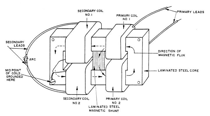
To reduce overall bulk, (size) and for reasons of lower cost manufacturing, the transformer's coils are designed to handle only 1/2 the terminal voltages. This applies to both primary and secondary. For one thing the coils themselves can be built with insulation that need handle only 1/2 the voltage stress — this saves money. Second, the overall bulk of the coil can be shaped to fit into a smaller sized case.
