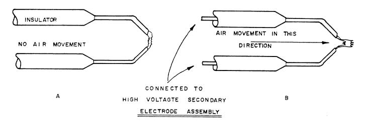
This demands more voltage to establish the arc and maintain it. To create a reasonable safety margin (to allow for conditions of low line voltage, dirty or leaky insulators on the draught tube electrodes), 10,000 volts is considered to be ideal for most burners in use. There are, of course, industrial and special burners that require higher burning rates and higher blast tube air velocities. For these 12,000 volts transformers and even higher ratings are used.
