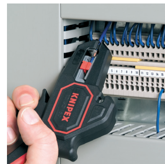
Stripping in confined areas
