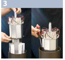
Replace acrylic lens\* and top cover, tighten top cap allen screw
